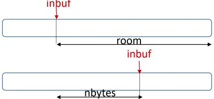
Read next piece of data (of size room) from fd into a computed place in buffer
