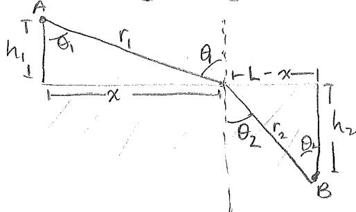
$\text{Time} = T = \frac{r_1}{v_1} + \frac{r_2}{v_2}$
